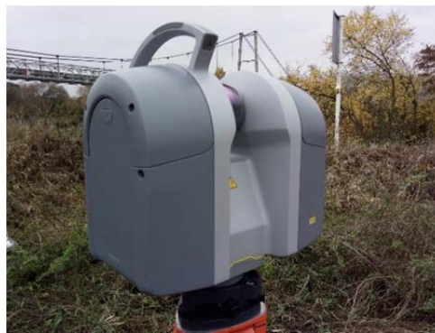
Fig. 8: Trimble TX8 scanner second attempt.
