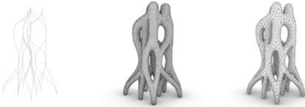
Fig.5 The piping process of the reticular line network and the re-meshed version of the tower
