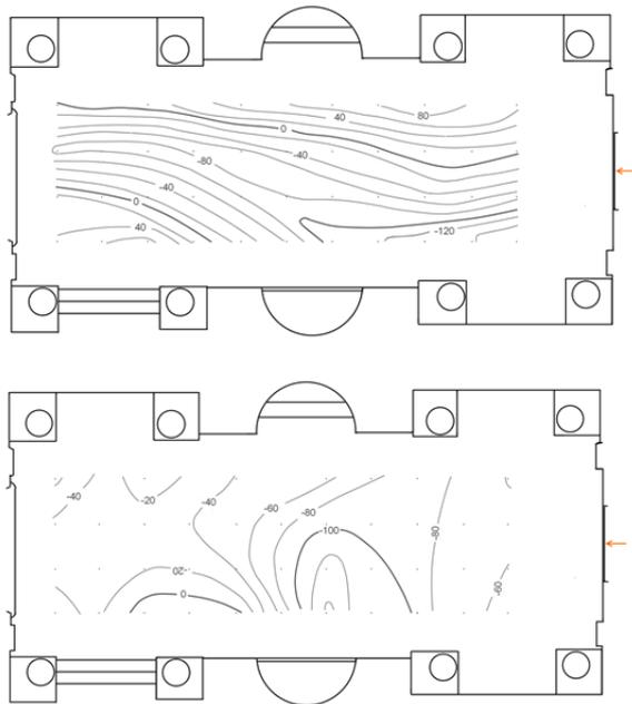
pic 3 a,b . Horizontal gradients of gravity  $W_{xz}$  (3a) and  $W_{yz}$  (3b) from variometer E-60, contour value 20 E.
