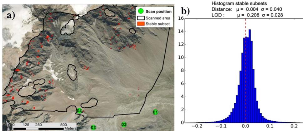
**Figure 1:** a) Scan setup and stable subsets used to assess the error budget b) histogram of the point cloud distance measurements in all stable subsets.
