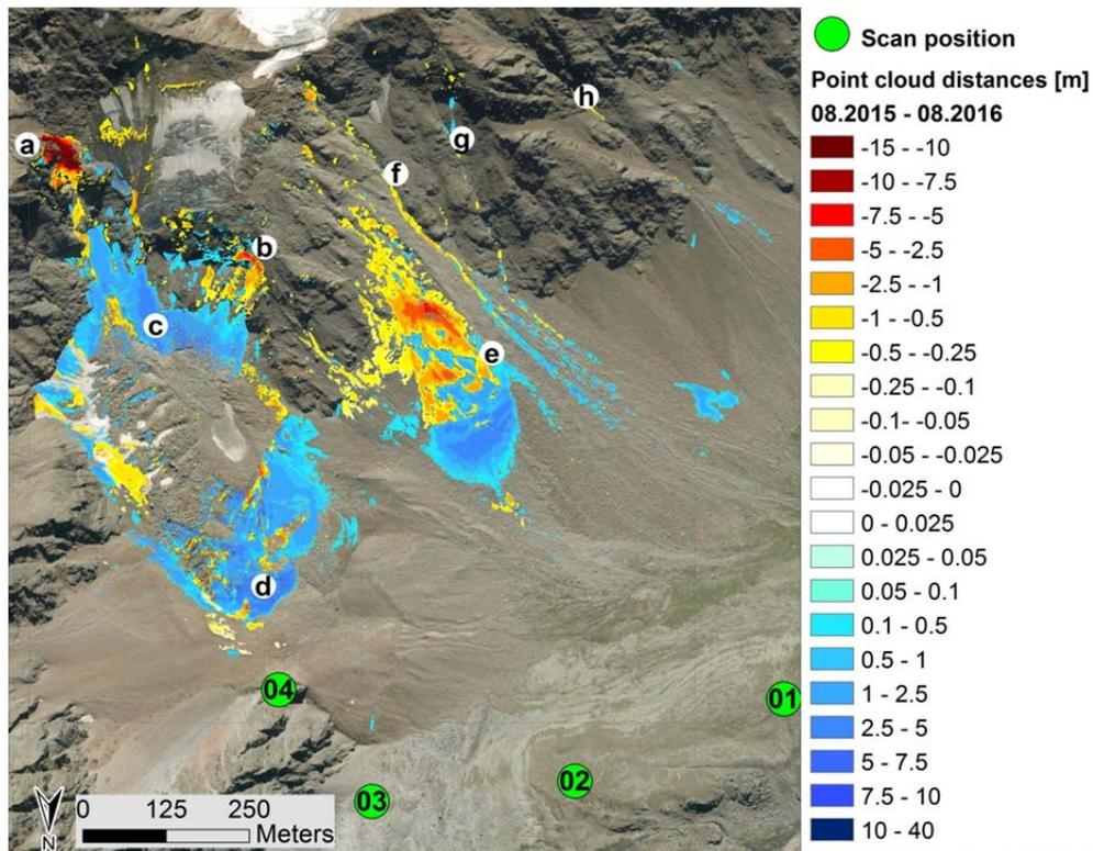
Figure 3: Point cloud distance measurements in areas automatically detected as changed. The characters a-h are described in the text.
