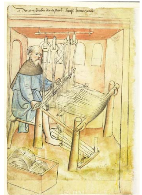
horizontal treadle loom Miniature taken from The House Book of the Mendelian Twelve Brothers Foundation in Nuremberg, 1437 AD
