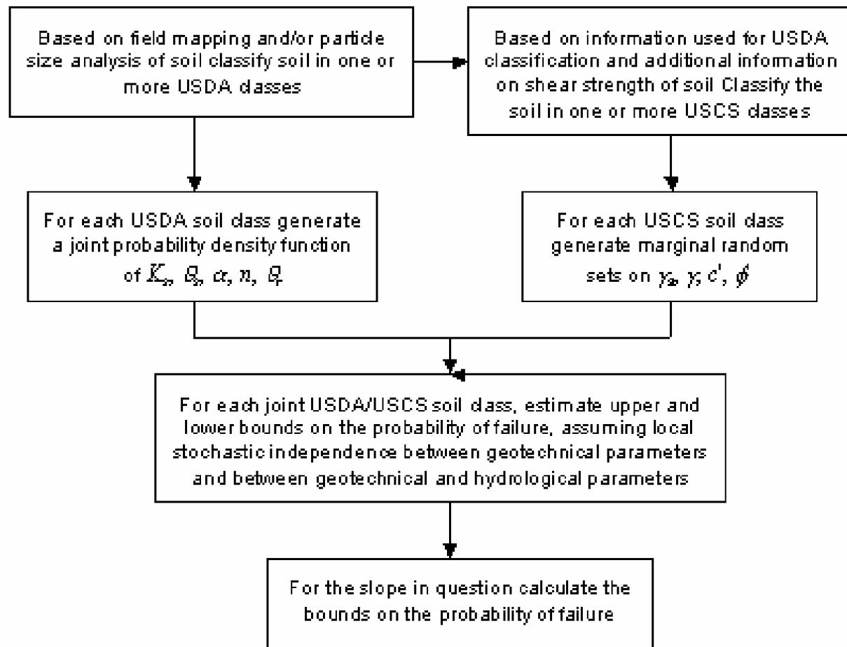
Suppose that the lower and upper bounds on the probability of the factor of safety exceeding some value  $x$  are written  $P_-(FoS > x)$  and  $P_+(FoS > x)$ , respectively, then the probability of slope failure  $P_f$  lies in the interval  $[P_-(FoS \leq 0), P_+(FoS \leq 0)]$ .
