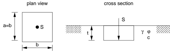
Figure 1: Bearing capacity example
