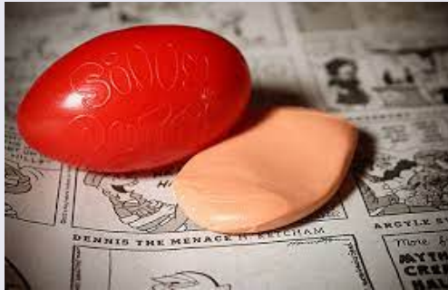
Silly putty which can flow, bounce or break depending on strain rate.
