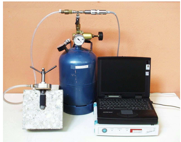
Fig.2: On-site test setup (Packer test)
