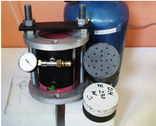
Fig. 1: Laboratory test setup (Disk test), the sample is not yet inserted in the cell
