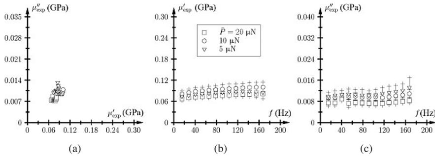
Fig. 5. (a) Cole–Cole diagram, mean values and standard deviation for (b) storage modulus  $\mu'_{\text{exp}}$  and (c) loss modulus  $\mu''_{\text{exp}}$  as a function of frequency for different values of  $\bar{P}$  (cono-spherical tip).
