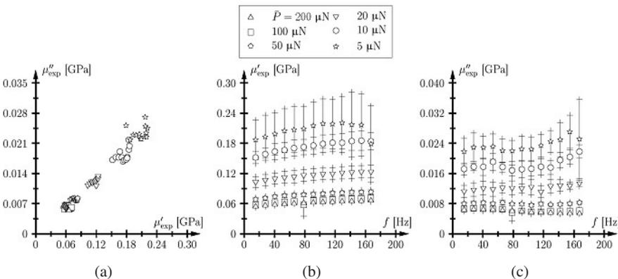
Fig. 4. (a) Cole–Cole diagram, mean values and standard deviation for (b) storage modulus  $\mu'_{exp}$  and (c) loss modulus  $\mu''_{exp}$  as a function of frequency for different values of  $\bar{P}$  (Berkovich tip).
