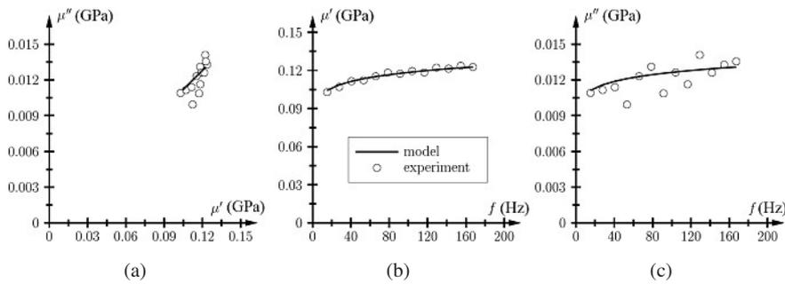
Fig. 6. Comparison of experimental results and model response obtained from parameter identification: (a) Cole–Cole diagram, (b) storage modulus  $\mu'$ , and (c) loss modulus  $\mu''$  (experimental data for  $\bar{P} = 20 \mu\text{N}$  and  $P_0 = 0.2 \mu\text{N}$ ).
