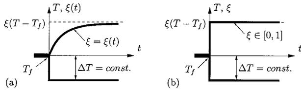
**Fig. 4.** Illustration of freezing kinetics: evolution of  $\xi$ : (a) obtained from linearly decreasing chemical affinity function and (b) adopted in proposed material model
