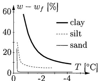
**Fig. 2.** Unfrozen water content  $w - w_f$  as function of  $T$  for different types of soil (Willams 2001) ( $w$ : water content of unfrozen soil;  $w_f$ : frozen water content)
