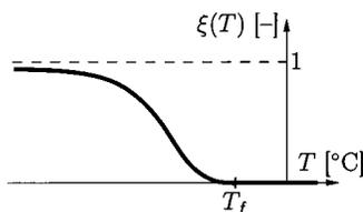
Fig. 9. Thermal freezing function  $\xi(T - T_f)$  characterized by  $\xi = 0$  at  $T = T_f$  and  $\xi \rightarrow 1$  for  $T \ll T_f$
