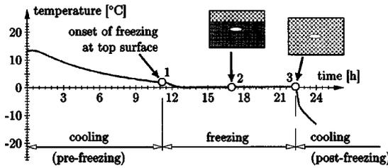
**Fig. 7.** Freezing experiments: typical temperature history monitored by temperature sensor B
