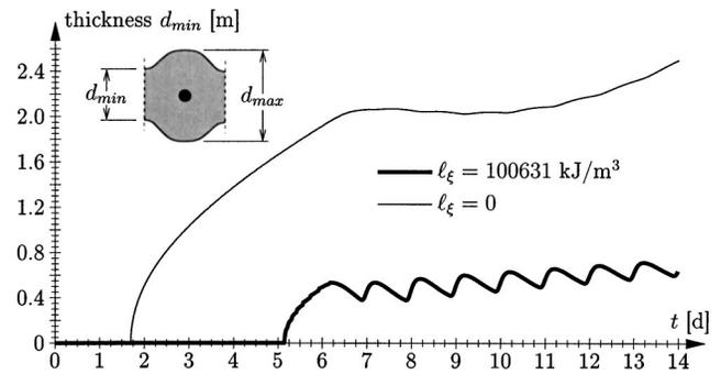
**Fig. 22.** Application: influence of latent heat  $\ell_{\xi}$  on evolution of minimum thickness  $d_{\min}$  of frozen-soil body
