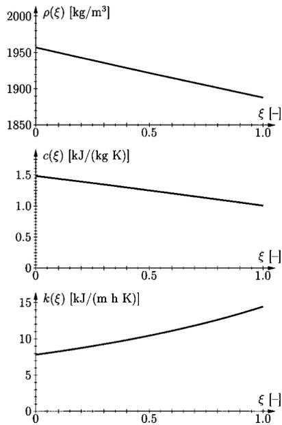
Fig. 8. Freezing experiments: thermal properties for freezing sand as function of  $\xi$
