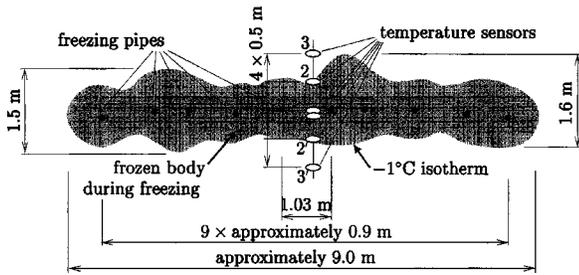
**Fig. 12.** Application: cross section of test Field V2 showing location of freezing pipes and temperature sensors
