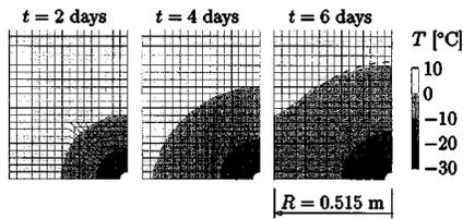
Fig. 17. Application: numerically obtained temperature distribution for different instants of time
