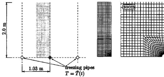
Fig. 15. Application: numerical model and finite-element discretization
