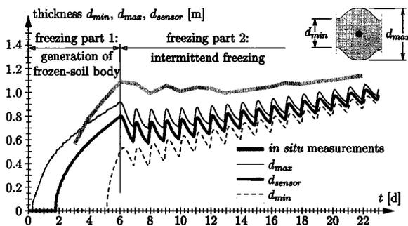
Fig. 18. Application: numerically obtained evolution of thickness of frozen-soil body characterized by  $T \leq -1^\circ\text{C}$
