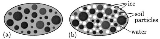
**Fig. 5.** On determination of thermal conductivity from continuum micromechanics: employed material representation of (a) unfrozen soil and (b) frozen soil
