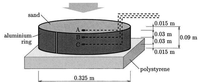
**Fig. 6.** Freezing experiments: experimental setup and geometric dimensions
