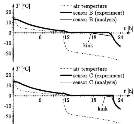
Fig. 11. Freezing experiment: measured temperature histories and results obtained from numerical analysis with  $\bar{T} = 0.2^\circ\text{C}$  and  $\alpha(\xi = 1) = 85 \text{ kJ}/(\text{m}^2 \text{ h K})$
