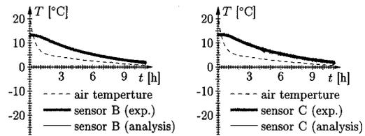
Fig. 10. Freezing experiments: measured temperature histories and results obtained from numerical analysis with  $\alpha = 300 \text{ kJ}/(\text{m}^2 \text{ h K})$
