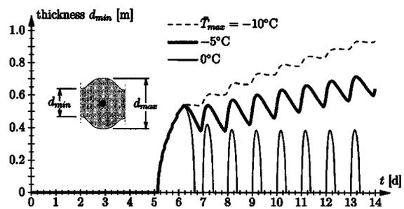
Fig. 20. Application: evolution of  $d_{\min}$  for different temperature levels  $\bar{T}_{\max}$  and  $\Delta t = 3$  h
