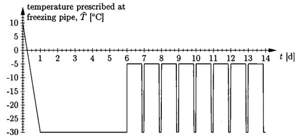
**Fig. 14.** Application: temperature history in freezing pipe employed in analysis
