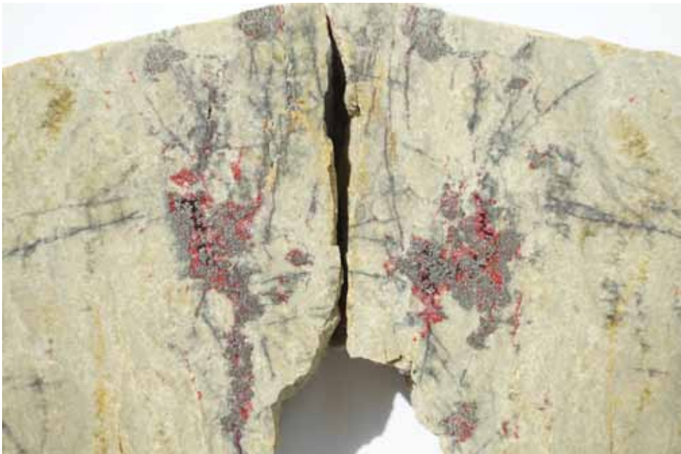
Figure 1. Two cut and polished samples of siderite ore (light-brownish) from „Steirischer Erzberg“. The cinnabar- (red) and pyrite- (metallic grains) bearing zones contains the Ni-sulfides. Width of photograph: ~10 cm.
