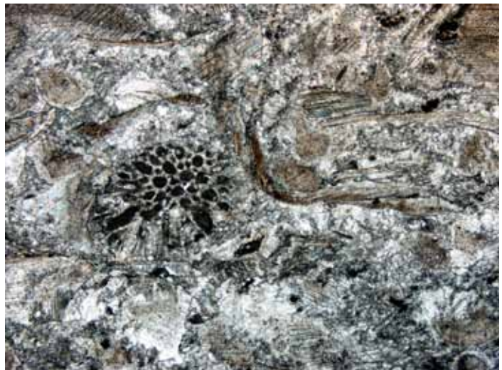
Figure 9: Thin section photograph of Steinsberger Kalk at the Lange Wand. The limestone is a crinoidal packstone to rudstone composed of abundant crinoid fragments and subordinate of brachiopod shells, bivalves and bryozoans. Plane light, width of photograph is 6.3 mm.
