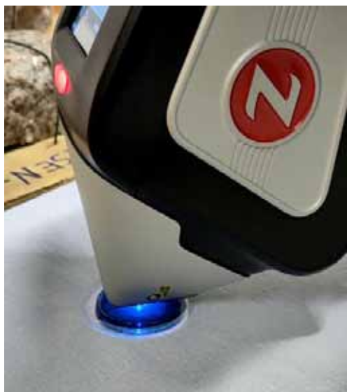
Fig. 1: pLIBS measurement on a fused bead containing Cu as dying agent.
