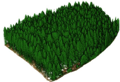
3D view of the UAV point cloud of a spruce stand.
