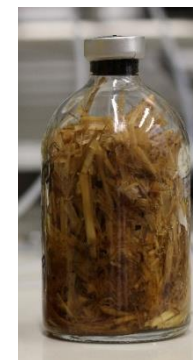
Batch reactor with straw (high load, HCL)
