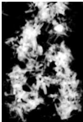
Figure 1: Synthetic B-rich tourmaline. Backscattered electron image, width: 6.5 \mu\text{m} .
