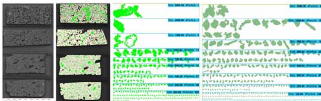
Figure 1: Example of the analysis of samples from La Palma volcanic eruptions in 2023. From left to right: (a) Total X-ray intensity map that highlights the potential different mineral phases in the sample; (b) AMICS Mineralogical classification that clearly identifies the phenocryst phases from the matrix; (c) size distribution of clinopyroxene phenocrysts; (d) size distribution of olivine phenocrysts.
