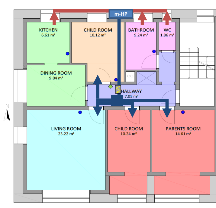
Fig. 3. Floor plan of the renovated flat in ground floor with a simplified scheme of ducting for ventilation and heat distribution [5]
