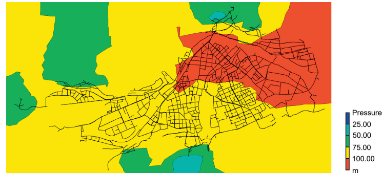
Fig. 2. Pressure distribution within the water supply network of the case study Innsbruck.
