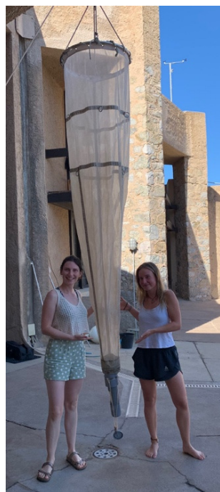
Figure 1: Hensen net. Conical net with a metal ring at the entry side and a collecting container at the ending side. Julia (on the left), 172 cm and Laura (on the right), 166 cm as size reference.
