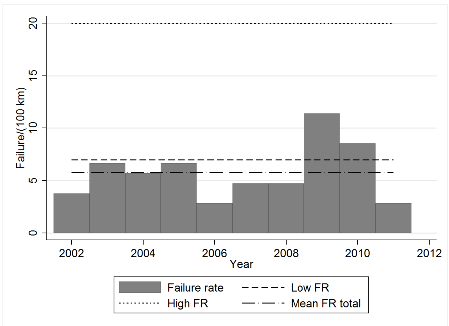
Figure 35: Failure rates for the water distribution pipes of case study 3
