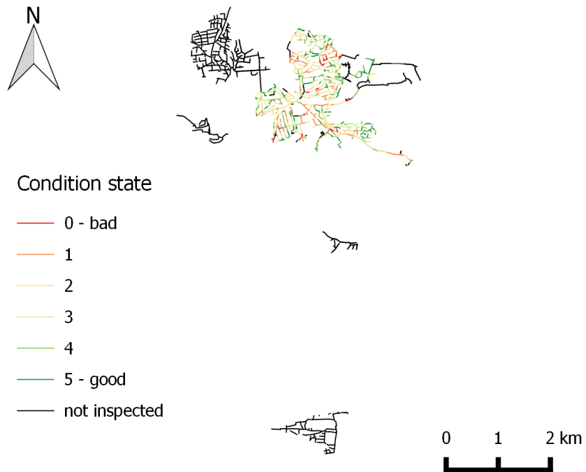
Figure 39: Condition states using DWA-M 149-3 (2007) of the urban drainage network of case study 3
