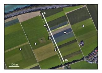
The proposed scintillometer path at Kolsass measuring 550 m from transmitter (Tx) to receiver (Rx). Eddy covariance stations are marked by a cross (existing station) and circles (additional stations). Aerial imagery from Google Earth.
