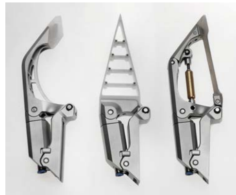
Figure 4: The three jaw modules a) Pincher b) Fish Fin (FFM) and c) Adaptive (AM)
