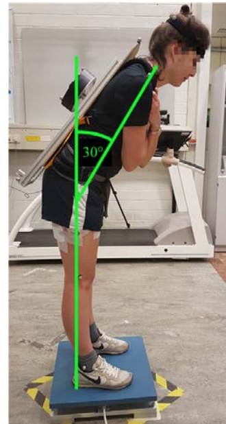
Figure 3: Trunk forward angle calculation
