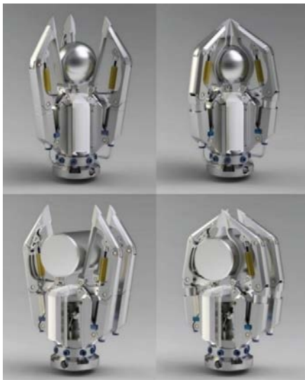
Figure 5: Grasping basic geometries with the adaptive jaw module
