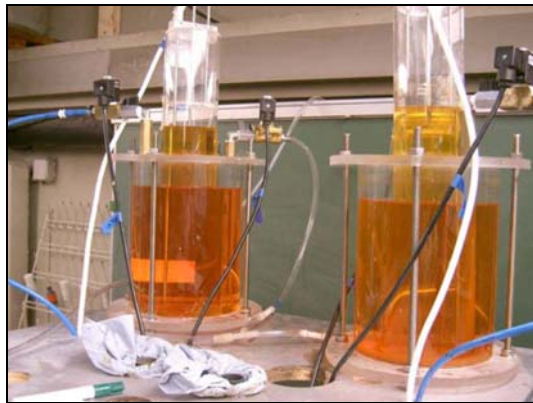
Figure 3-2 Gas meters on top of the lab digesters
