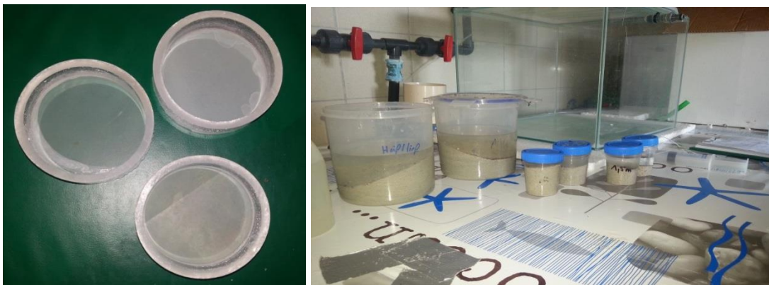
Figure 1: Filters of different mesh sizes and sand samples of the different sample depths
