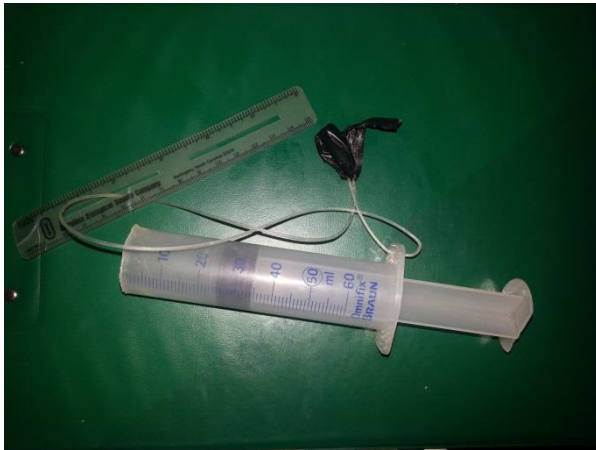
Figure 2: Core-sampler for consistent sample amounts
