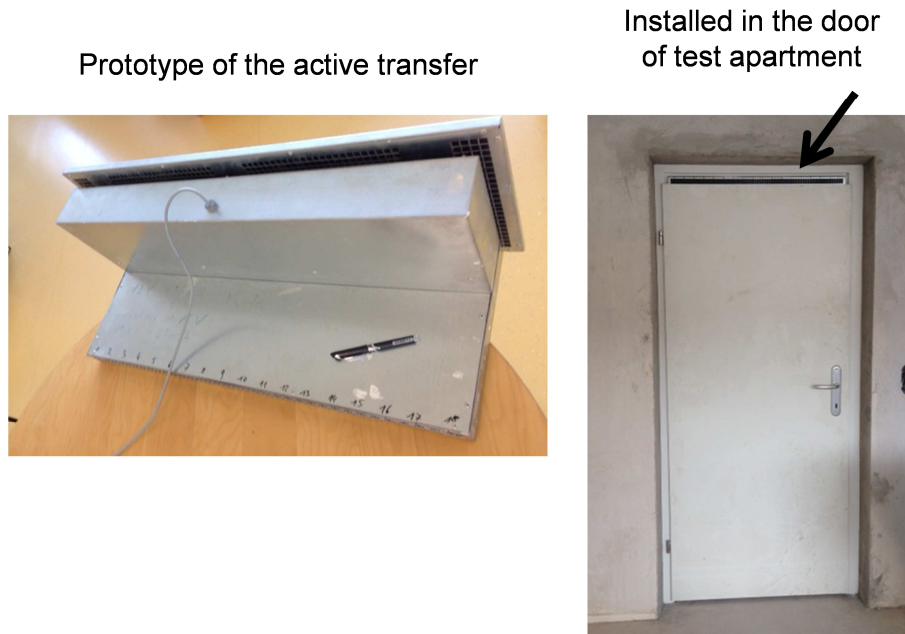
Figure 48: Photographs of the prototype of active transfer (left). View from the room with the outlet of the active transfer (right)
