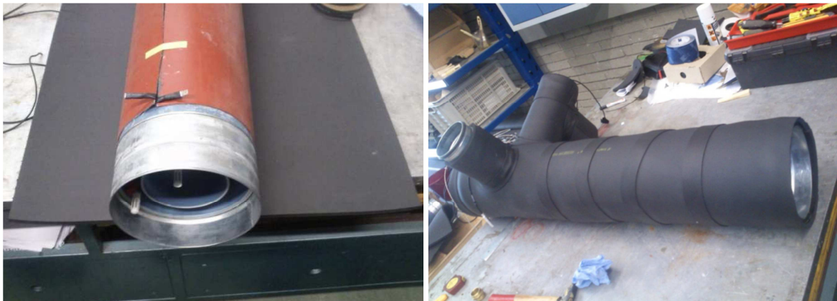
Figure 76: Left: heating foil wrapped on the prototype of a coaxial duct. Right: the whole duct is then wrapped by insulating and vapor impermeable material.
