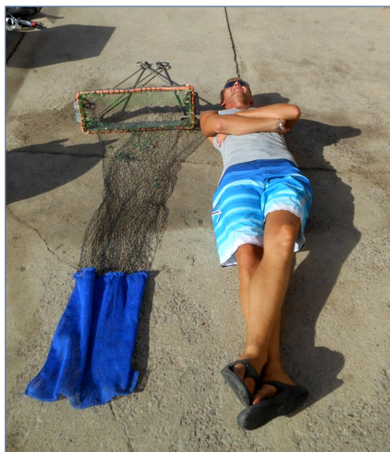
Fig.5: Length relationship between the Dredge and BSc Benedikt Zeindl. The aperture was 40mm in the upper part and 5 mm in the lower part. The bucket opening was 60 cm.
