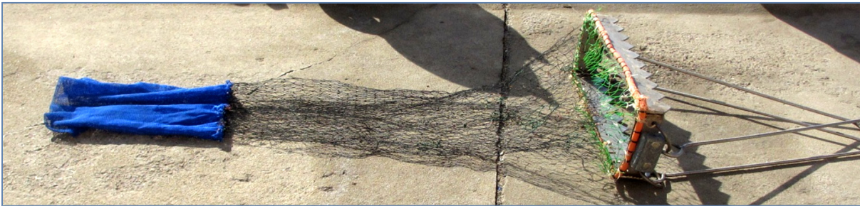
Fig.5: The dredge that was used to sample the Corraligène.
