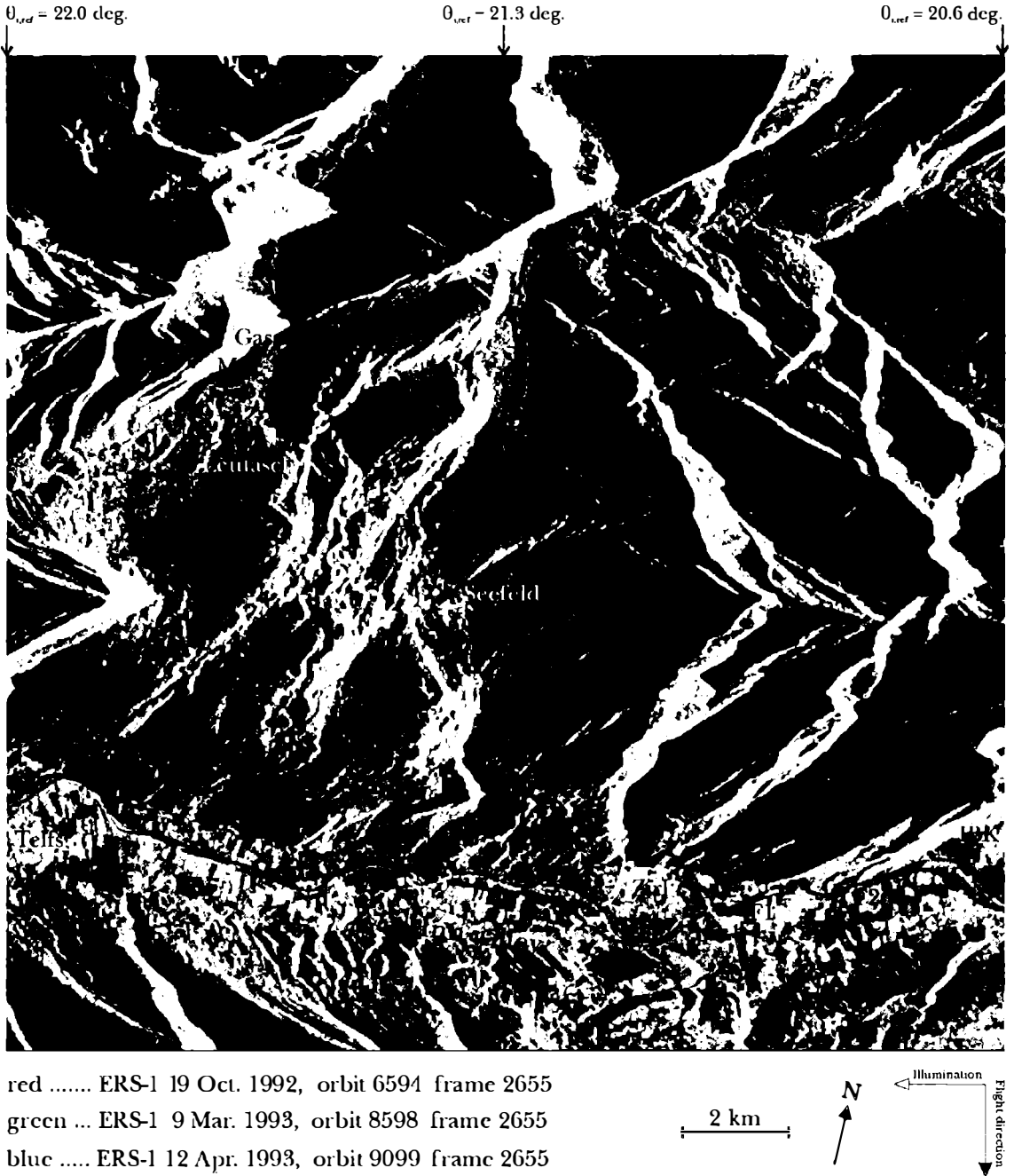
Figure 7.22: Multitemporal repeat pass ERS-1 image of track 437, frame 2655 of 19 October 1992 (red), 9 March 1993 (green), 12 April 1993 (blue). Sites used for signature analysis are marked by F1, F2, M1, M2, C1. At the top of the figure the variation the local incidence angle \theta_i along the direction of radar illumination on a flat area is specified.
