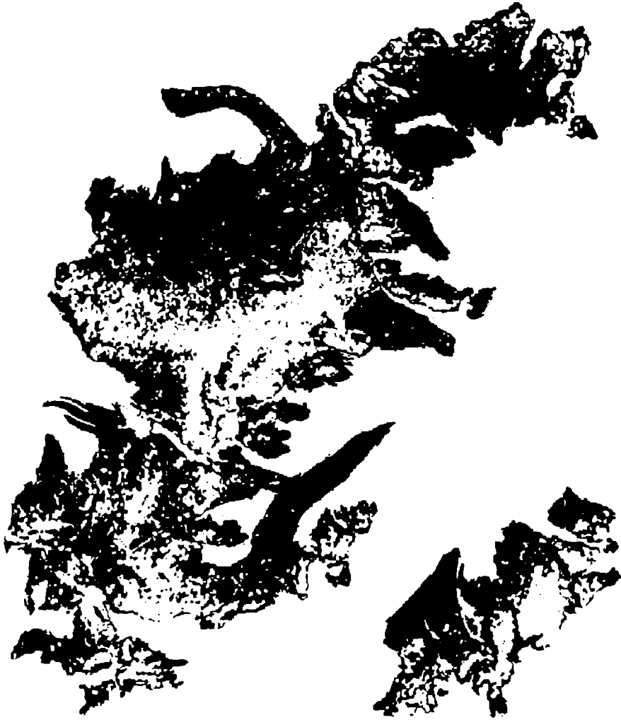
Figure 11.8: Extent of firn areas (white) and ablation areas (black) on glaciers in Ötztal, derived from X-SAR data from 3 October 1994. Layover and shadow areas are shown in medium grey, ice free areas in light grey.
