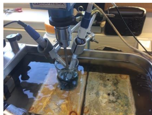
Figure 10. Measuring the potential and the pH in the Cu-tartrate solution
