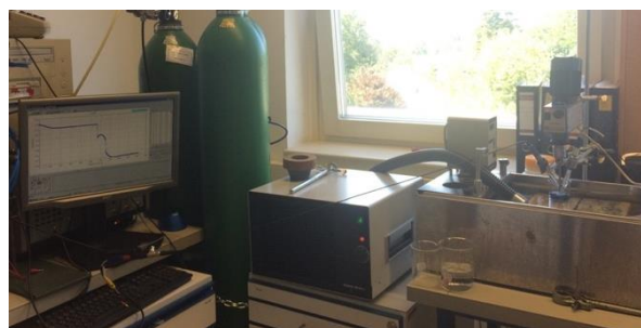
Figure 9. Experimental set-up. From left to right: computer, cooler device, beaker with the fabric placed at the stirrer and immersed in Cu-tartrate solution.
