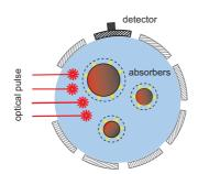
Figure 1.1: ILLUSTRATION OF PAT. Electromagnetic pulses are sent into the investigated object and induce acoustic waves. The acoustic waves are measured with ultrasound detectors on the boundary of the object and are used to recover an image of the object.
