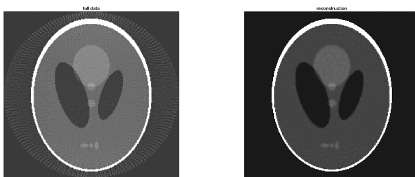
Figure 6.1: Reconstruction via FBP from 200 sensors (left) and reconstruction from 66 Bernoulli measurements after 1000 iterations using the proposed method (right).
