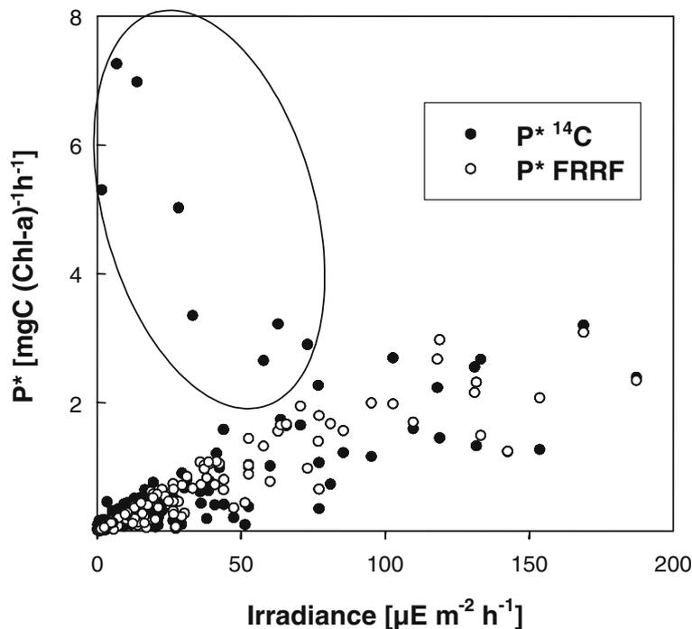
Figure 5. Relationship between all estimates of FRRF- and  $^{14}\text{C}$ -productivity in  $\text{mgC (Chl-}a\text{)}^{-1} \text{ h}^{-1}$  and total available radiation in  $\mu\text{Einst m}^{-2} \text{ s}^{-1}$ .  $^{14}\text{C}$ -based measurements during *P. rubescens* blooms are marked. As discussed in the text, these values are underestimated by FRRF due to the excitation band-width of the cyanobacterial species, which is not exactly in the spectrum of the Fluorometer.
