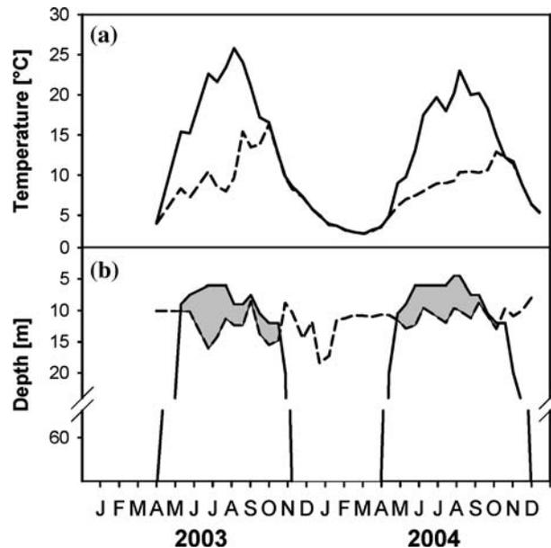
Figure 2. Physical variability during the sampling period 2003/2004. (a) surface water temperature (solid line) and metalimnetic temperature (dashed line) in °C; (b) mixing depth ( $Z_{\text{mix}}$ , solid line) and euphotic zone ( $Z_{\text{eu}}$ , dashed line) in m. The shaded area indicates the stratified period.
