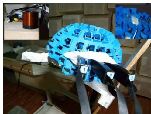
Fig. 1. Participant helmet with three dual-axis OPMs inserted over the auditory cortex. Insets show (top left) the coil used for generating the trigger pulses and (top right) the triple-axis accelerometer attached at the apex of the helmet.
