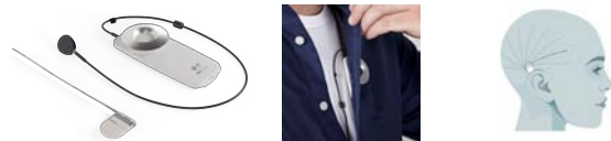
Fig. 1: The measurement setup analysed in this work. Left: UNEEG medical's SubQ implant and 24/7 EEG SubQ Recorder. Center: Demonstration of recorder placement in the upper chest area. Right: Subcutaneous implant and lead positioning. Images rights are with UNEEG medical A/S [5].
