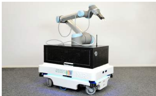
Fig. 1. Mobile manipulator CHIMERA from JOANNEUM RESEARCH
