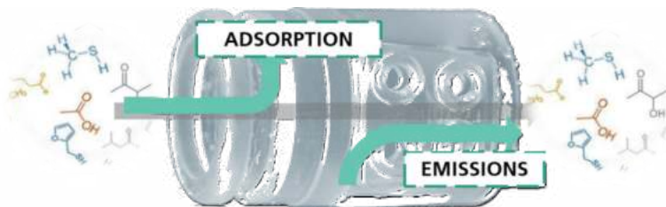
Figure 2: Schematic depicting the purging of a breath sampling mouthpiece with breath-relevant volatiles or clean, humid air to assess the degree of compound uptake of the former or emissions into the latter, as is of relevance for potential confounding effects for breath samples.
