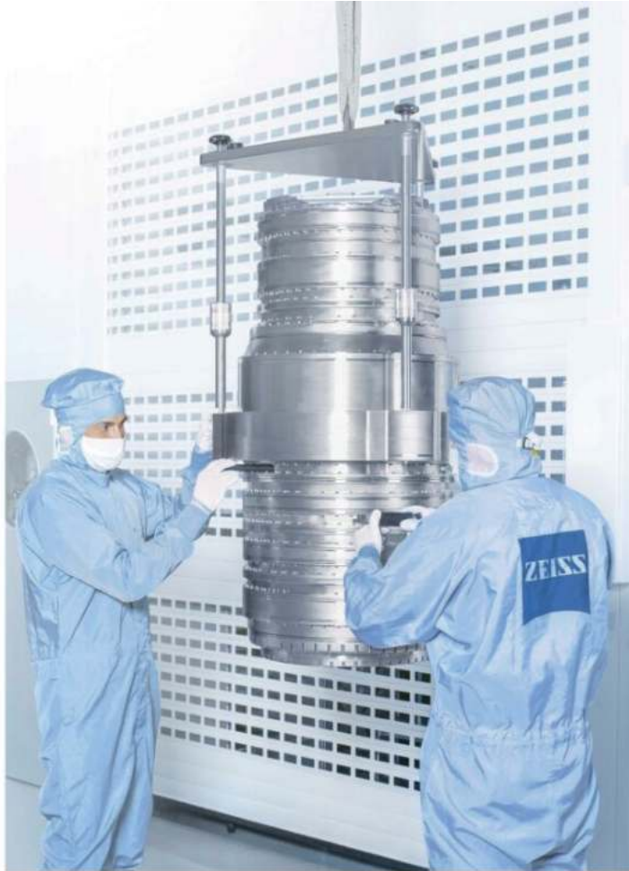
Figure 1: Two ZEISS employees handling a DUV photo lithography optic. The optics final quality control for volatile contaminants is carried out with PTR-MS
