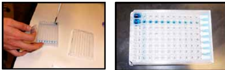
Figure 3: Photographs illustrating scale and micro-channel flow (left to right). Once the source well is primed, the dye is seen to migrate from left to right.
