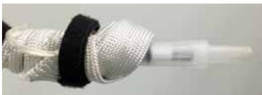
Figure 1: Direct Mouth-Space (DMOS) sampling setup: BET mouthpiece coupled to the heated sampling and dilution lance
