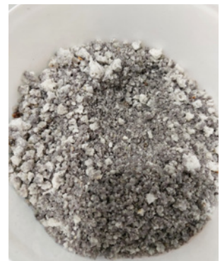
Figure 2: Cupola furnace slag to substitute the cement content in briquettes
