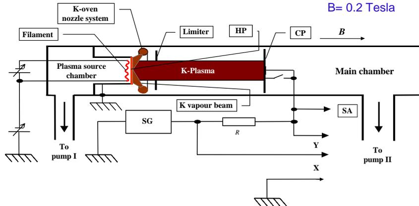
HP = hot plate, CP = cold plate, SG = signal generator, SA = spectrum analyzer
