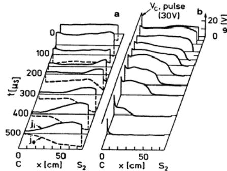
Temporal evolution of the ion and electron density profiles (LHS up – ion, down – electron) and of the plasma potential profile (RHS) during one period of the PRI.
