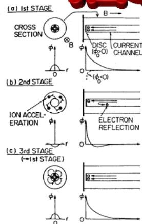
Schematic of the temporal evolution of ions and of the plasma potential profile inside the current channel during one period of the EICI.
