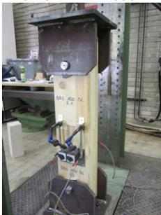
Figure 6: Built tensile test
