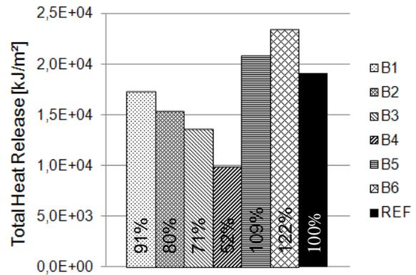
Figure 2: Total heat release after 600 seconds (THR<sub>600</sub>)
