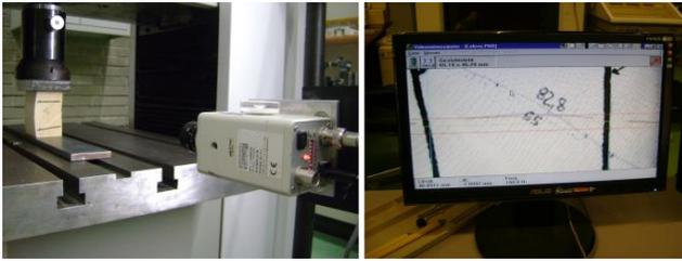
**Figure 2:** Measurement of deformations with the Videodensimeter ME46
