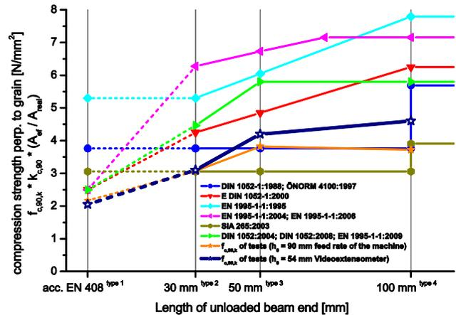
**Figure 3:** Comparison of the test results with calculations of different codes and standards.
