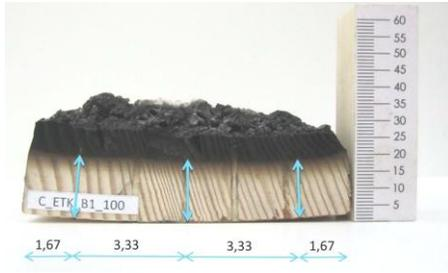
**Figure 2:** Measuring positions for the determination of wood char
