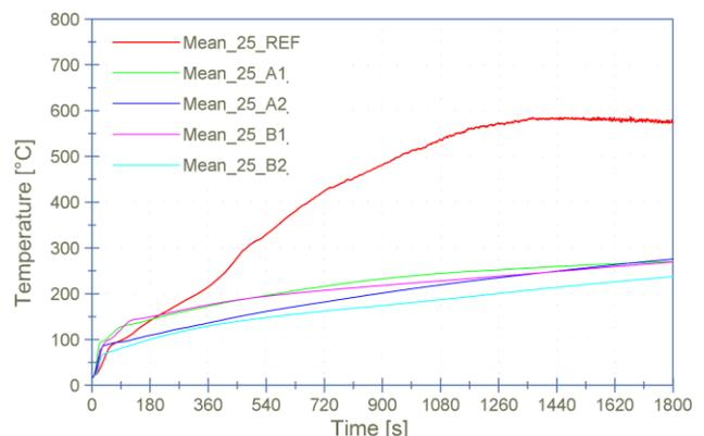
**Figure 4:** Temperature measured at -1 mm from the coated surface at the irradiance level at 25 kW/m<sup>2</sup>
