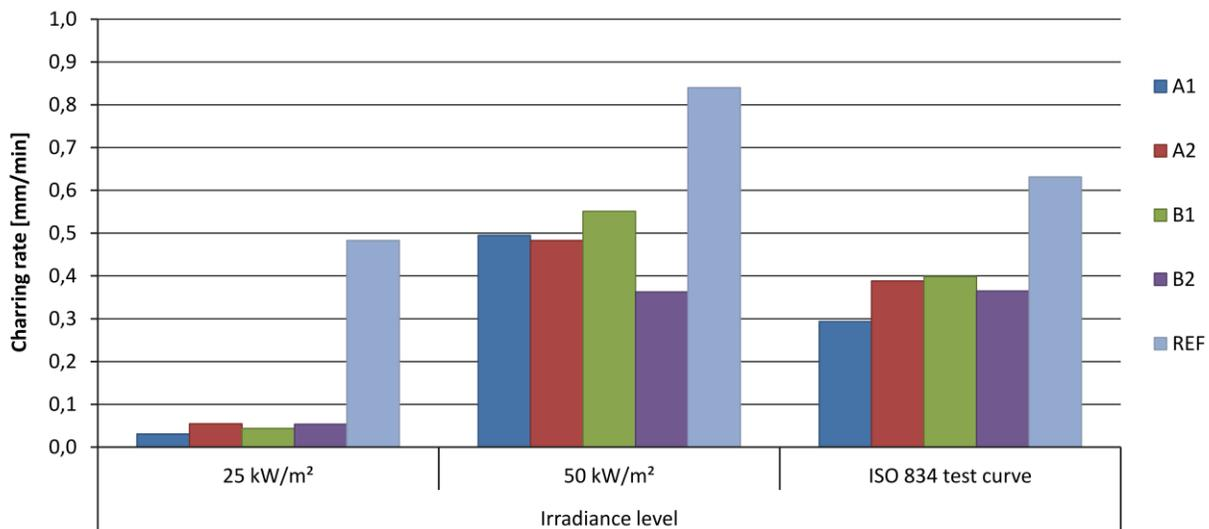
**Figure 3:** Charring rates of intumescent coated Norway spruce and uncoated reference material at different irradiance intensities tested with the cone calorimeter
