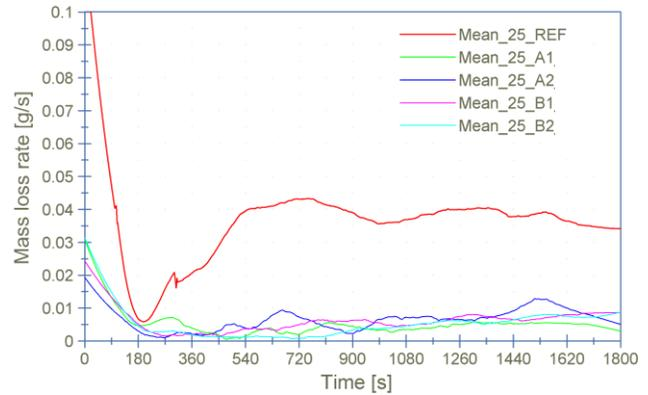
**Figure 7:** Mass loss rate at the irradiance level at 25 kW/m<sup>2</sup>
