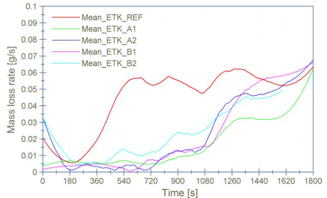
**Figure 9:** Mass loss rate at the irradiance level acc. the ISO 834 test curve
