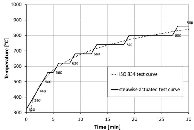
**Figure 1:** Temperature regulation steps for the irradiation level according to the ISO 834 standard test curve [11]
