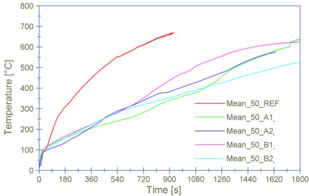
**Figure 5:** Temperature measured at -1 mm from the coated surface at the irradiation level at 50 kW/m<sup>2</sup>
