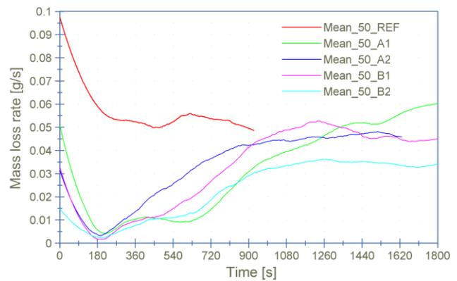
**Figure 8:** Mass loss rate at the irradiance level at 50 kW/m<sup>2</sup>
