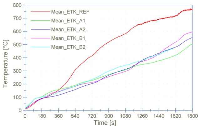
**Figure 6:** Temperature measured at -1 mm from the surface at the irradiation intensity of the ISO 834 test curve
