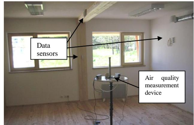
**Figure 2:** Realized wooden building module inside of the framing and clay module during air quality measurements
