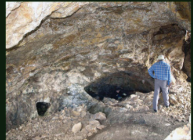
Ancient copper mine with fire-setting, in part reworked by blasting. Knappenkuchl/Navis. Photo: K.-P. Martinek
