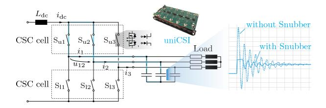
**Background:** Modern drive systems increasingly employ wide-bandgap semiconductors, enabling very fast switching transients. As a result, issues caused by high dv/dt and di/dt become critical. This project focuses on the design of a novel snubber circuit tailored for current source converters, aiming to suppress overvoltage and enable current control with high di/dt demands that were previously difficult to achieve.
