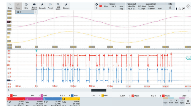
FIGURE 17: Simultaneously power and data transfer: In the upper half of the image, the currents on the primary and secondary sides were measured, while in the lower half of the image, the CAN bus signal on the primary and secondary sides was measured.
