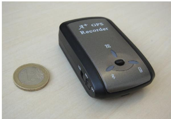
Fig. A1. GPS Satellite Logger Used During Taxi Rides
