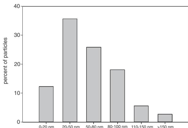
Fig. 2. Size distribution (%) of TiO<sub>2</sub>NP in Milli-Q water determined by TEM,  $n = 449$ .
