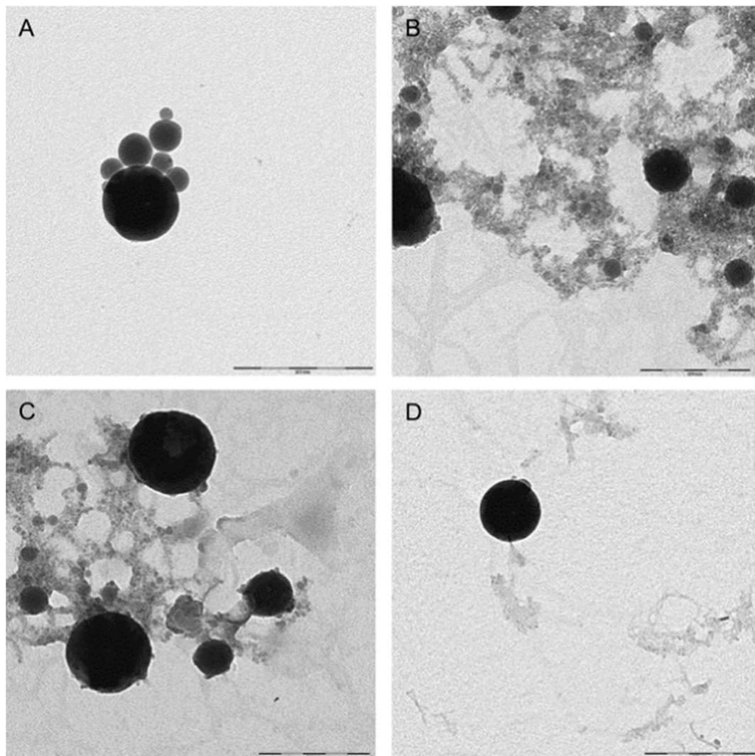
Fig. 3. Typical TEM images of TiO<sub>2</sub>NP in A) Milli-Q water, B) water from Lake Björklinge, C) Lake Erken and D) Lake Siggefora. Scale bars: 200 nm.
