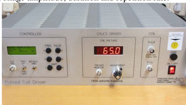
Figure 1. Home-built control unit for adjusting the parameters (pulse length, voltage and repetition rate) of the CRUCS valve.
