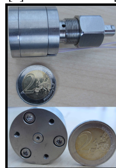
Figure 2. Front and Side View of the CRUCS Valve with Visualisation of size
