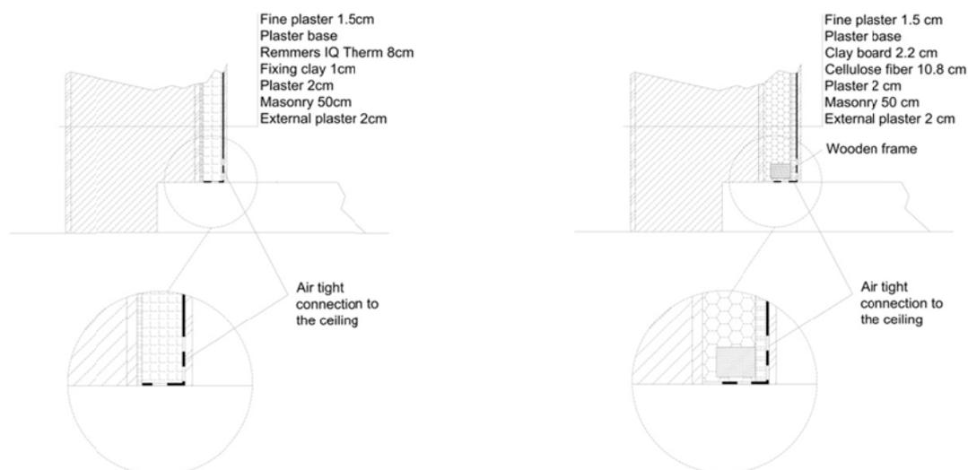
**Figure 1:** PU-foam insulation in combination with capillary active clay (left), Cellulose fiber and clay boards (right)
