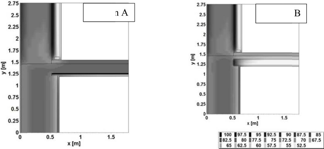
**Figure 3:** Moisture distribution (RH [%]) in the wall ceiling junction after five years (test room 2, cellulose type 1)
