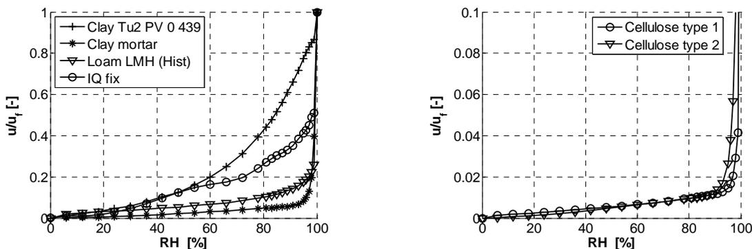
**Figure 4:** Normalized water retention curves for different Clays (left) and Celluloses (right)
