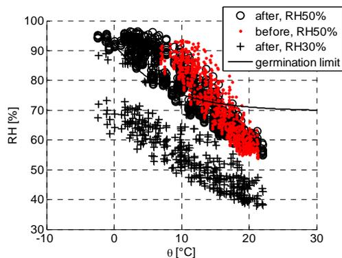
**Figure 7:** Mould germination, results before and after the insulation application with 50% and 30% internal RH. Section B, room 2
