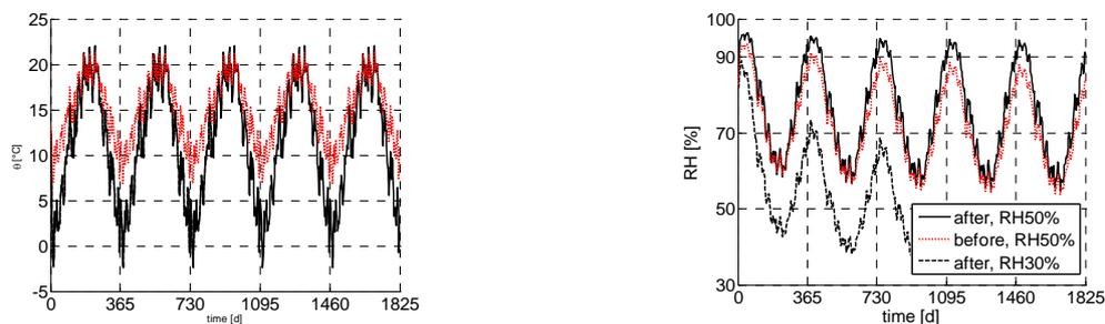
**Figure 6:** Temperature (left) and relative humidity (right) evolutions before and after the insulation application with 50% and 30% internal RH. Section B, room 2
