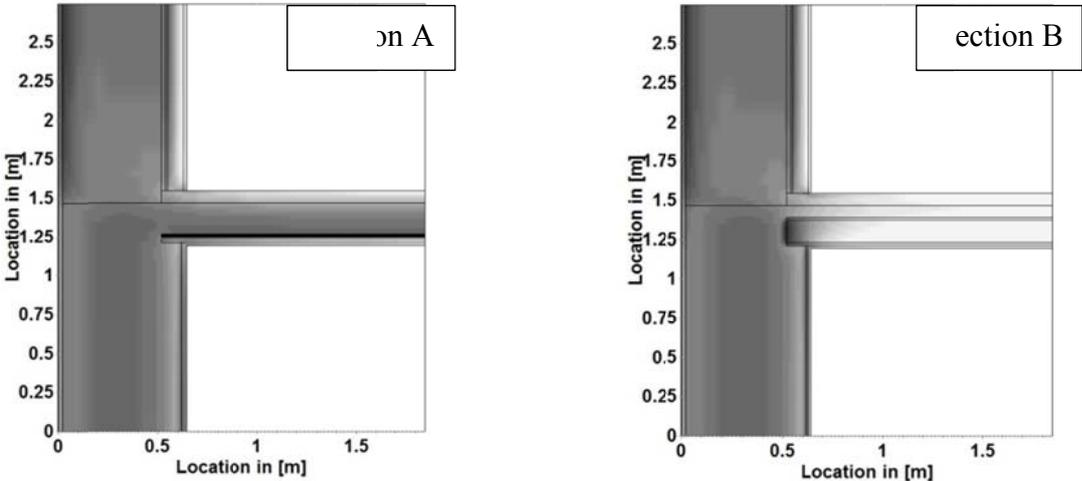
**Figure 2:** Moisture distribution (RH [%]) in the wall ceiling junction after five years (test room 1, Remmer system, Clay Tu2 PV 0 439 as fixing material).
