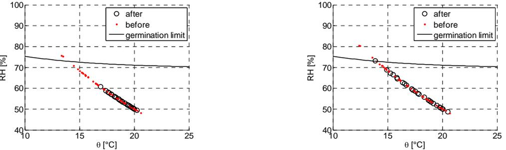
**Figure 10:** Mould germination limit section A (left) and section B (right), room 2
