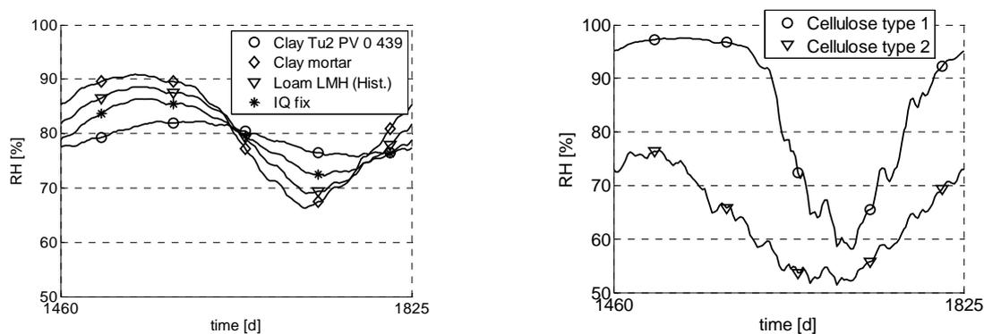
**Figure 5:** Relative humidity evolution at the wall-insulation interface. Left Test room 1 (Remmer system), right: test room 2 (cellulose)
